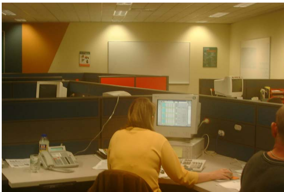
Figure 5. The screen on the workstation is far too dark so that the luminance contrast between the screen and the VDU is excessive.
