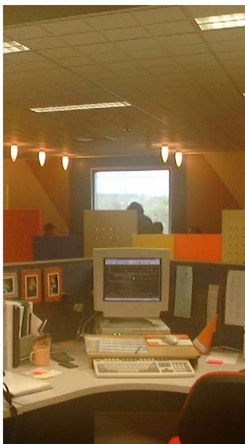
Figure 7. The window glare is located directly above the VDU giving a much higher surround luminance than the screen. The decorative lights are also bright small sources that act as distractions and effect the adaptation
