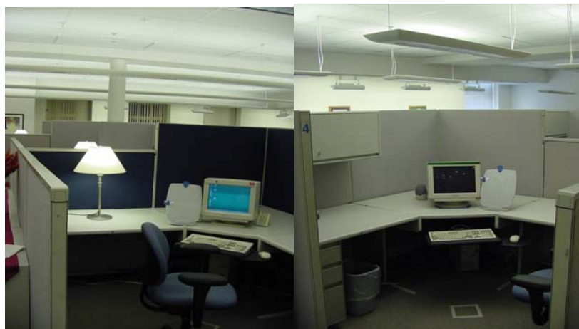
Figure 3. Cubicles used in the field simulation study (Boyce et al, 2003b and 2006) equipped with a switchable desk lamp (left) or a pendent luminaire that had a dimmable downward component. The difference in cubicle wall reflectance was balanced across both types of control.
